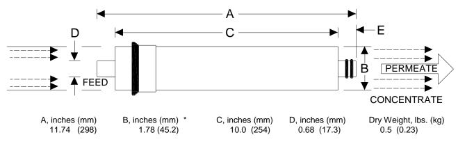
Core tube extension: E = 0.86" (21.8 mm)
