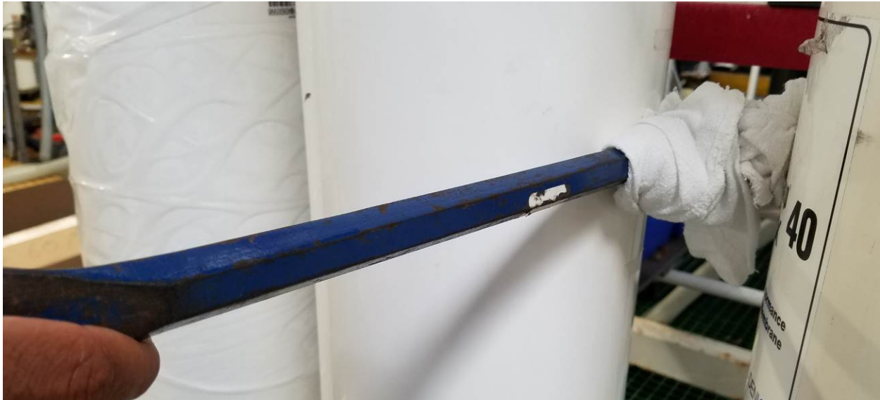
Figure 3: Crowbar with padding to separate modules.
