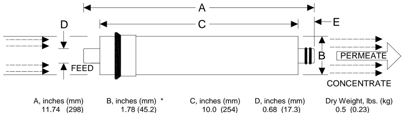
**Core tube extension: E = 0.86" (21.8 mm)**
