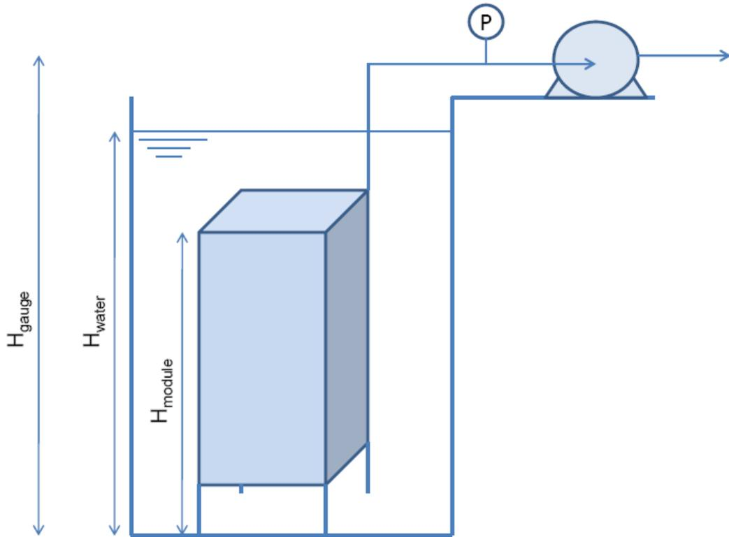
**Figure 1** Filtrate pump above the water level
