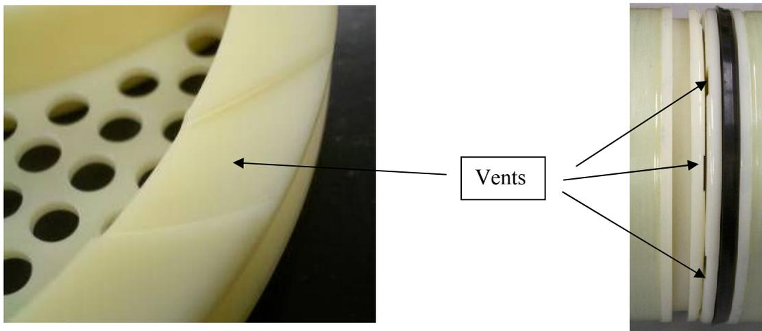
The added feature of vents provided in the new seal carrier designs will ensure that air can be readily removed from the annular gap between the outside of the element and the pressure vessel wall. This ensures rapid pressure equalization between the inside and outside of the spiral element. As a result, aggressive operation will be much less likely to cause damage, such as bursting of the FRP shell.
