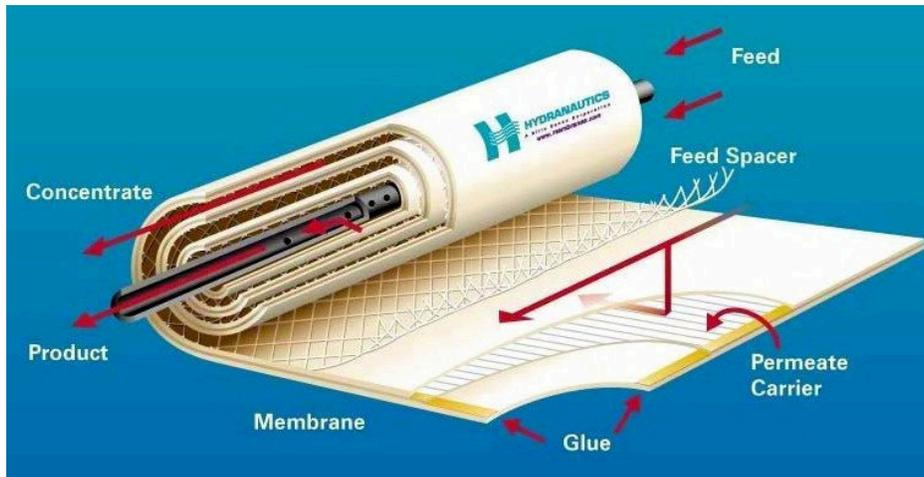
**Membrane Leaf Adhesives:** Improved adhesives have been developed which allow easier processing of the element, automation of the glue lines for improved quality and available active membrane surface area in RO element construction, improved chemical resistance at higher and lower pH, as well as stability at higher temperatures.
