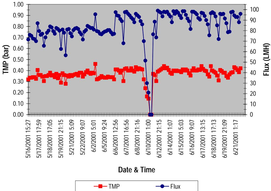
Figure 5: HYDRAcap TMP & Flux vs. Time
