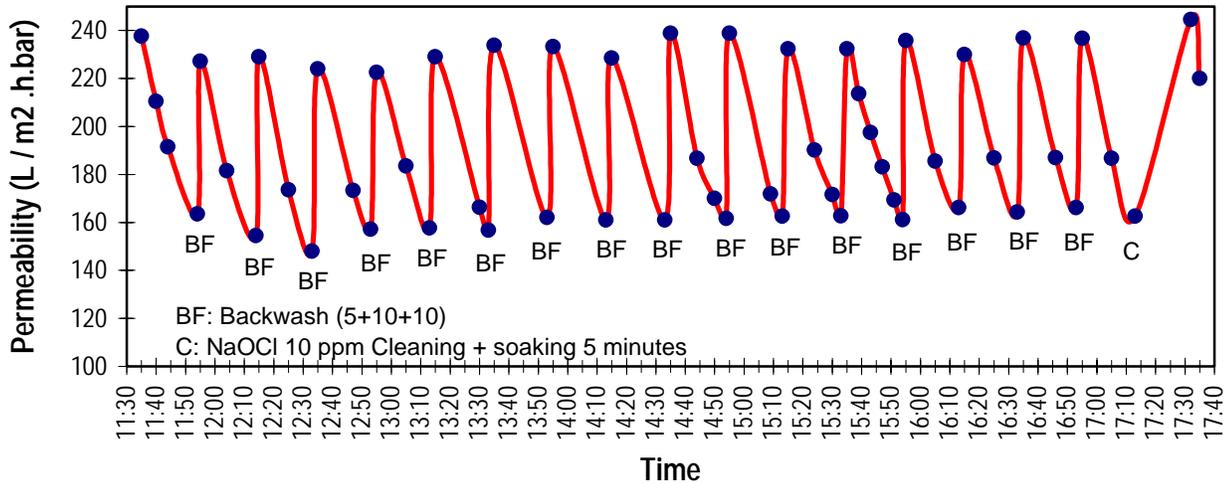
Figure 4: Backwash sequence during pilot test
