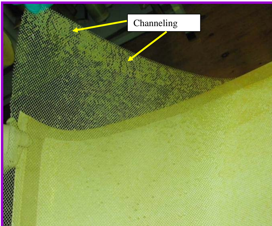
Figure 4 Fouled feedspacer from used element
