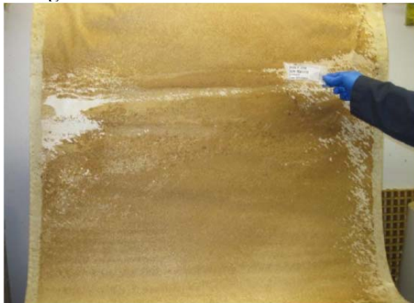
Figure 5 – Foulant on membrane sheet
