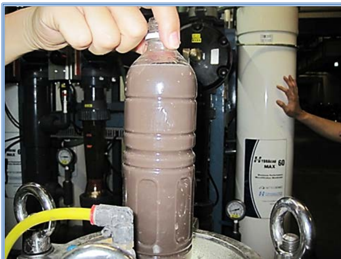
Figure 1: Feed Water Sample - Turbidity = 1100 NTU
