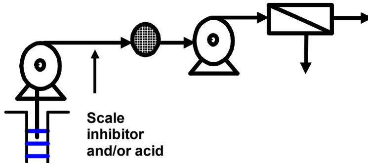
Figure 6. Configuration of brackish plant treating well water
