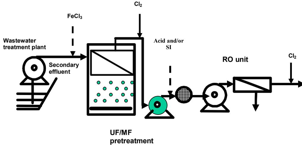
Figure 7. Configuration of wastewater reclamation plant using membrane pretreatment
