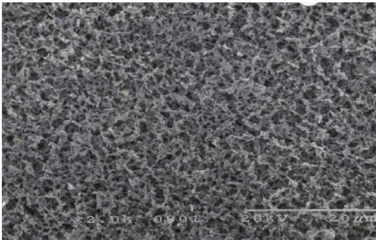
Figure 1 SEM image of clean SDI filter pad
