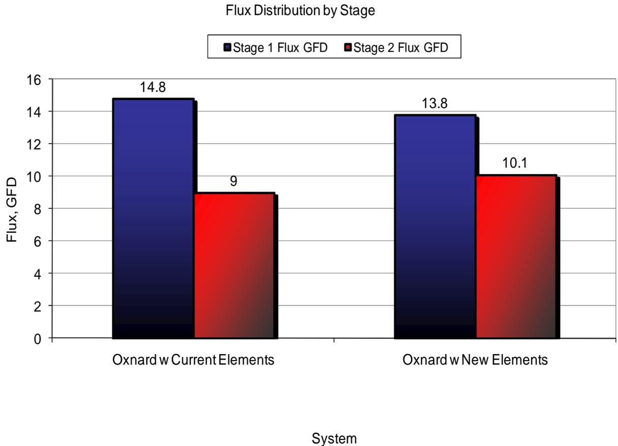
**Figure 2 Flux distribution between stage 1 and stage 2 for the Oxnard BWRO with current elements and with new, thicker brine spacer elements.**
