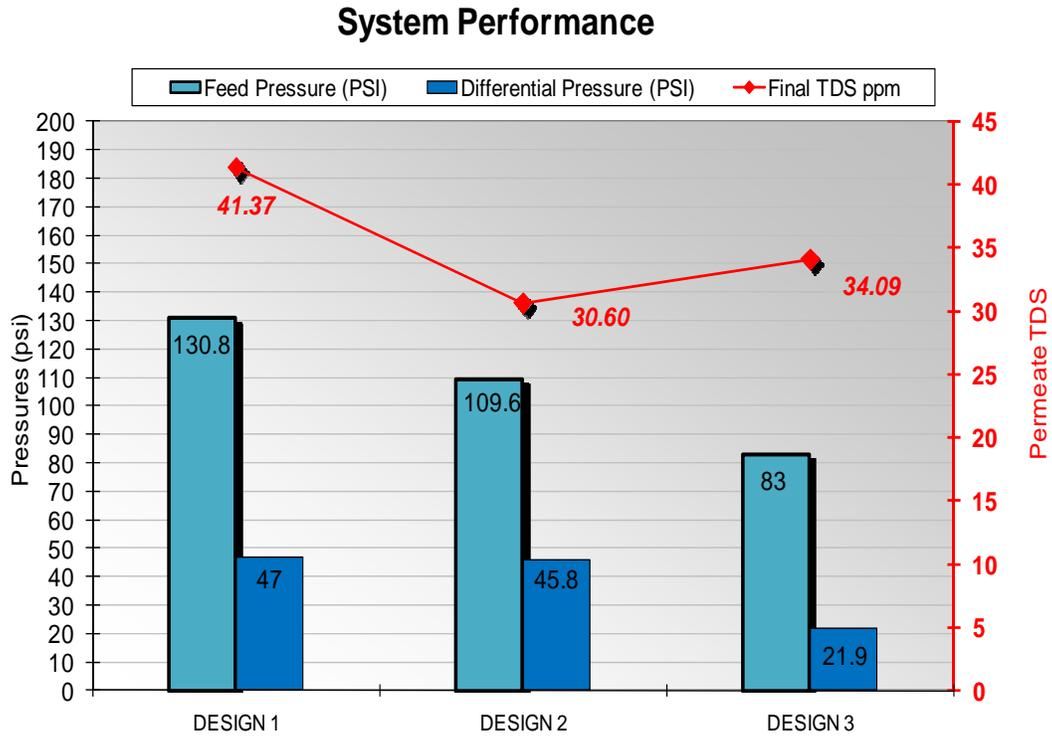
**Figure 3** Feed Pressures, Differential Pressures, and Permeate TDS of three different BWRO designs
