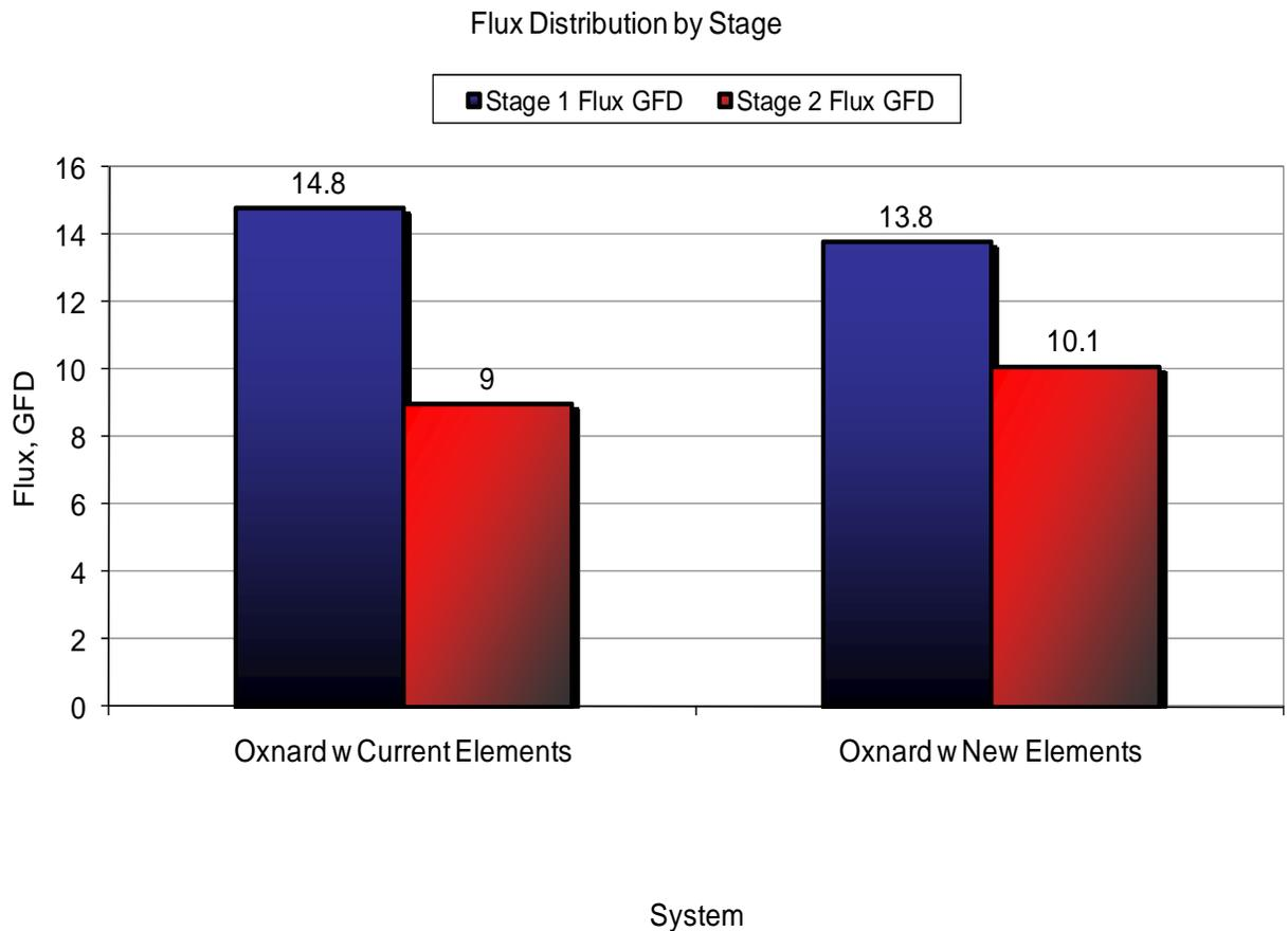
**Figure 2 Flux distribution between stage 1 and stage 2 for the Oxnard BWRO with current elements and with new, thicker brine spacer elements.**
