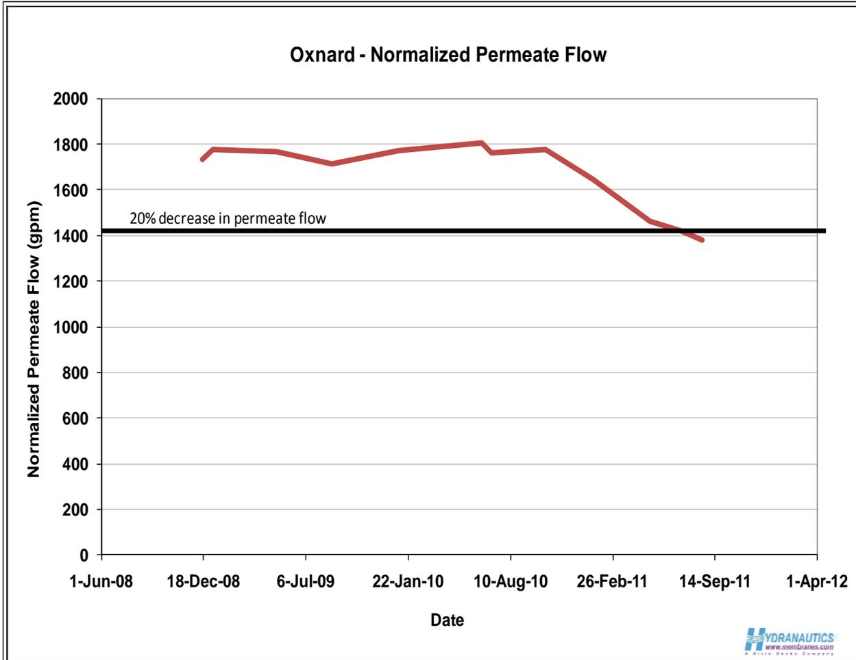
**Figure 5:** Oxnard’s normalized permeate flow during 3 years of operation
