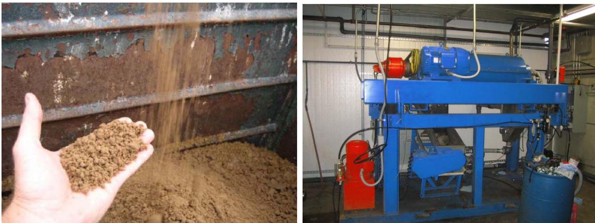
**Figure 8. Dewatered Sludge by Decanter Centrifuge and Centrifuge at Stone Brew Co. WWTP**
