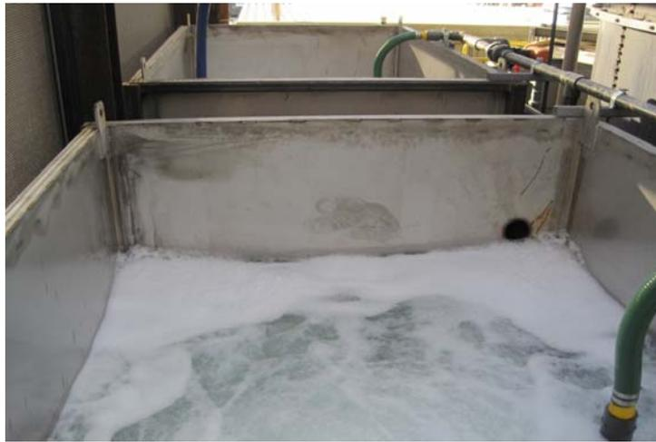
**Figure 3. Membrane Tanks during Clean Water Testing of Modules**
