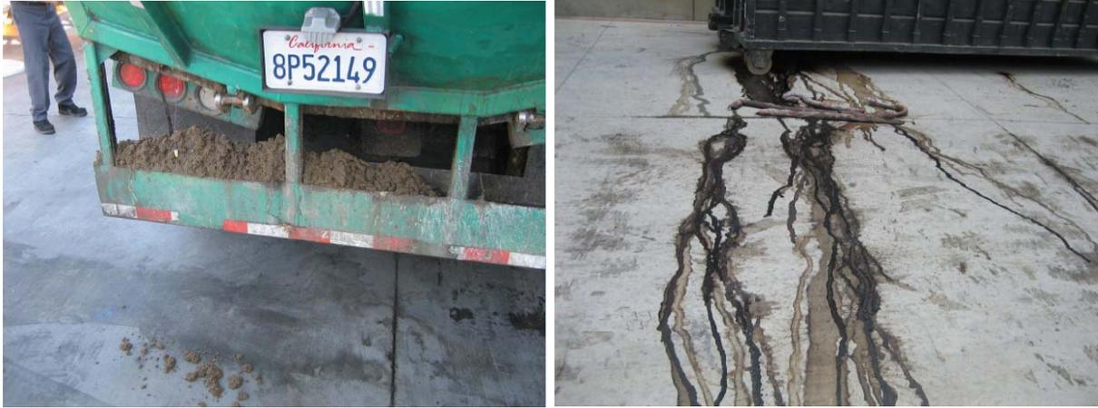
**Figure 7. Dewatered Sludge by Screw Press at Stone Brew Co. WWTP**
