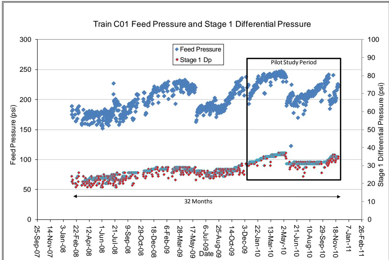
**Figure 3.** Three years of RO feed pressures and first stage differential pressures (Train C 01).
