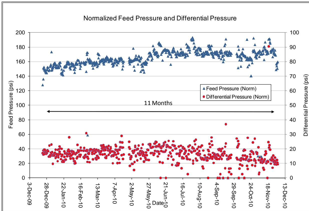
**Figure 2.** Eleven months of normalized feed pressure and differential pressure using the improved energy saving elements in a single pilot vessel attached to the first stage of Train C01.
