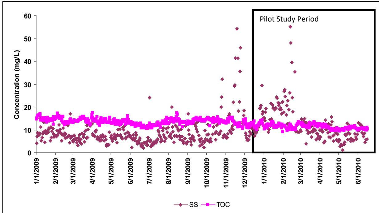
**Figure 4.** Suspended solids and TOC in feed to the MF membrane pretreatment.
