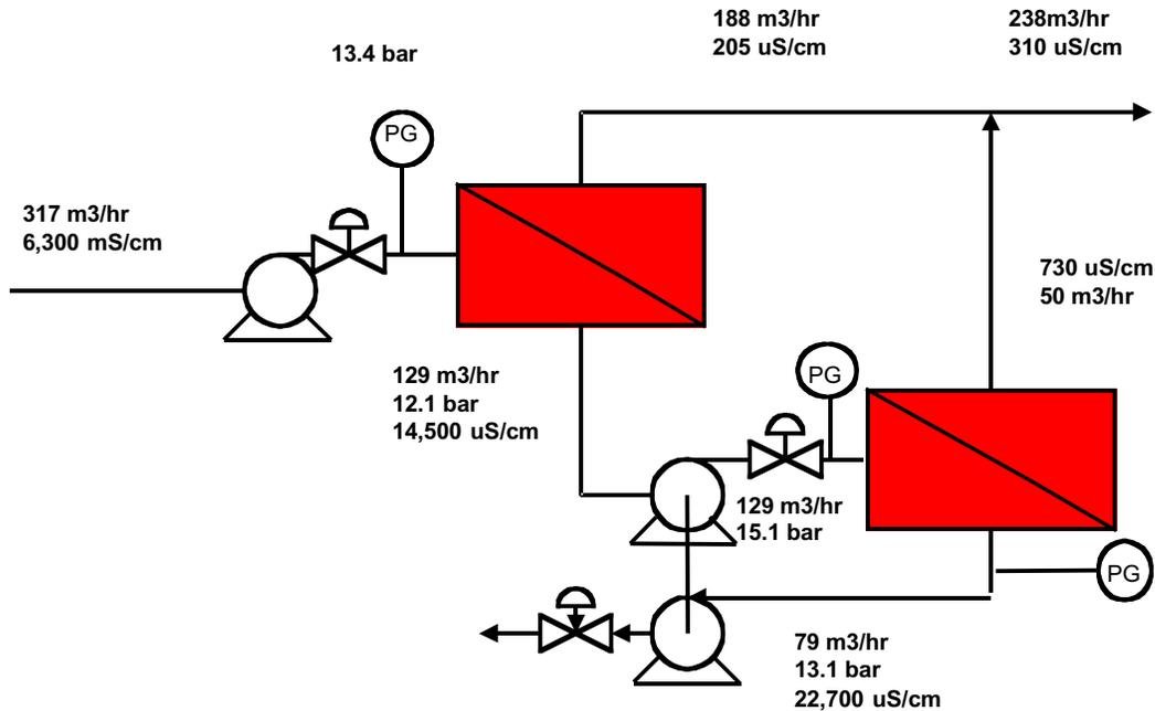
Flow diagram of a RO unit equipped with ESPA membrane elements at the Jupiter plant
