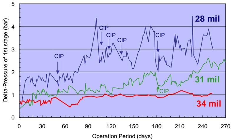
**Figure 1.** Performance of RO elements with different brine spacer thickness operating on high fouling feed water with SDI between 4 and 5.
