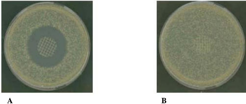
**Figure 2.** Bacterial growth after five days of incubation in colon bacillus on A) chemically enhanced spacer B) conventional spacer
