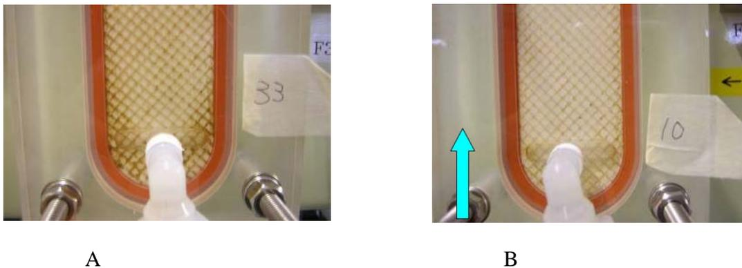
**Figure 3.** Biofouling on A) conventional spacer and B) biospacer after one month of continuous exposure to 0.5 L/min stream of waste water.
