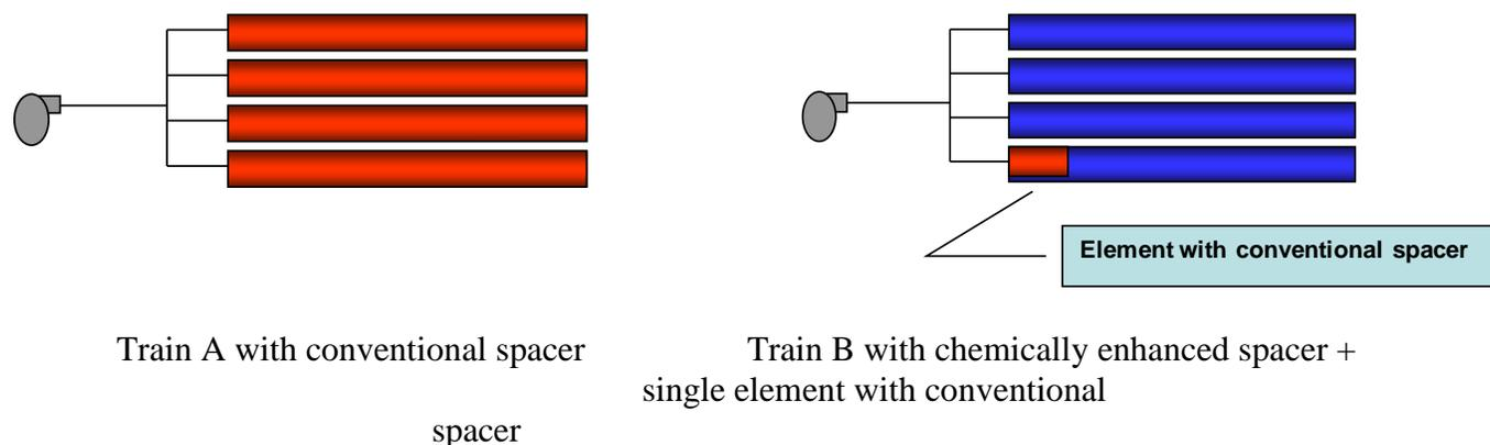
**Figure 4.** Two single stage trains with four vessels and six elements per vessel. Each train is running at 55% recovery and flux of 10 gfd. Train A is loaded with elements with 32 mil conventional spacer. Train B is loaded with elements with 32 mil chemically enhanced feed spacer and a single element with conventional spacer.
