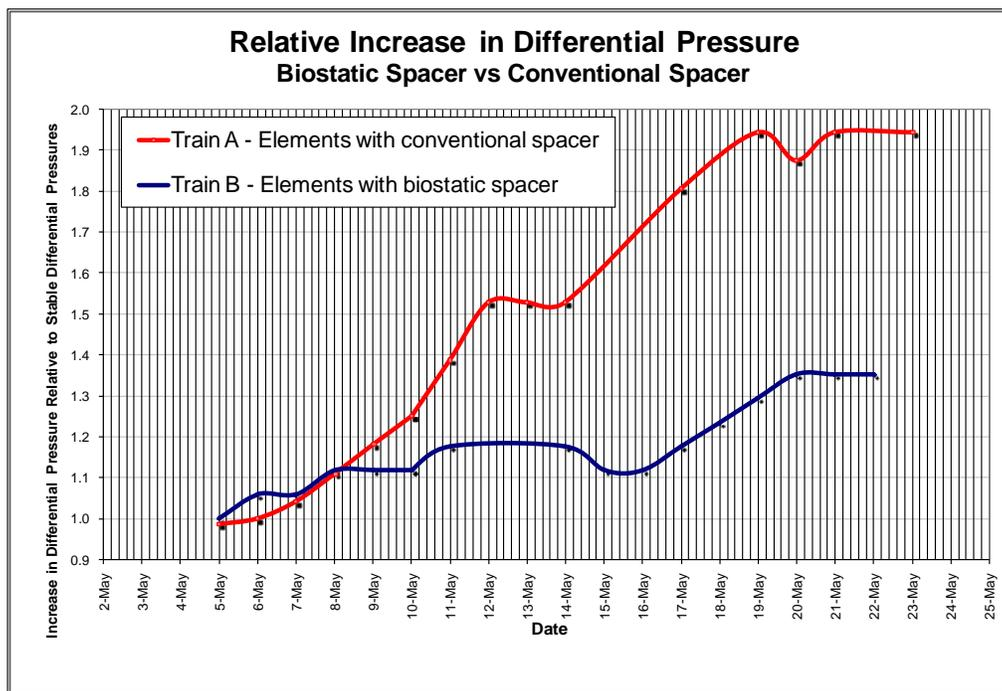
**Figure 5.** Relative increase in differential pressure of two RO trains running side by side during a severe biofouling event. Train A (red) operated with conventional spacer elements while Train B (blue) operated with a chemically enhanced spacer elements.
