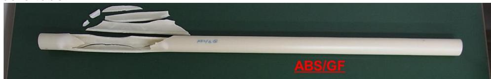
Permeate core tube collapse and mechanical failure.
