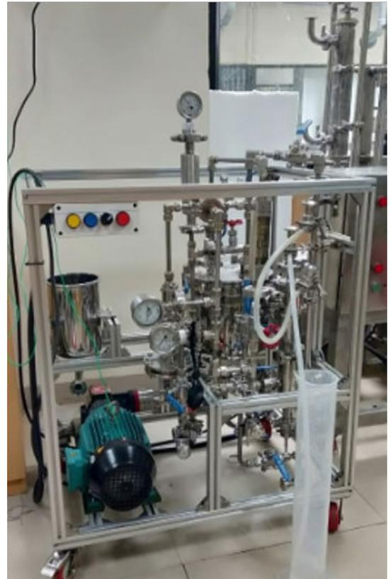
Figure 2: Picture of the lab-scale NF test unit
