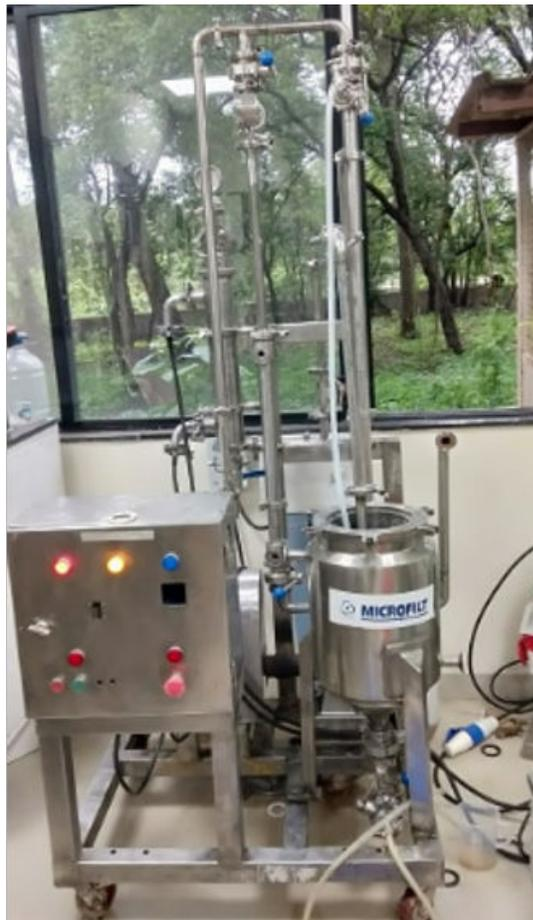
Figure 1: Picture of the lab-scale MF test unit
