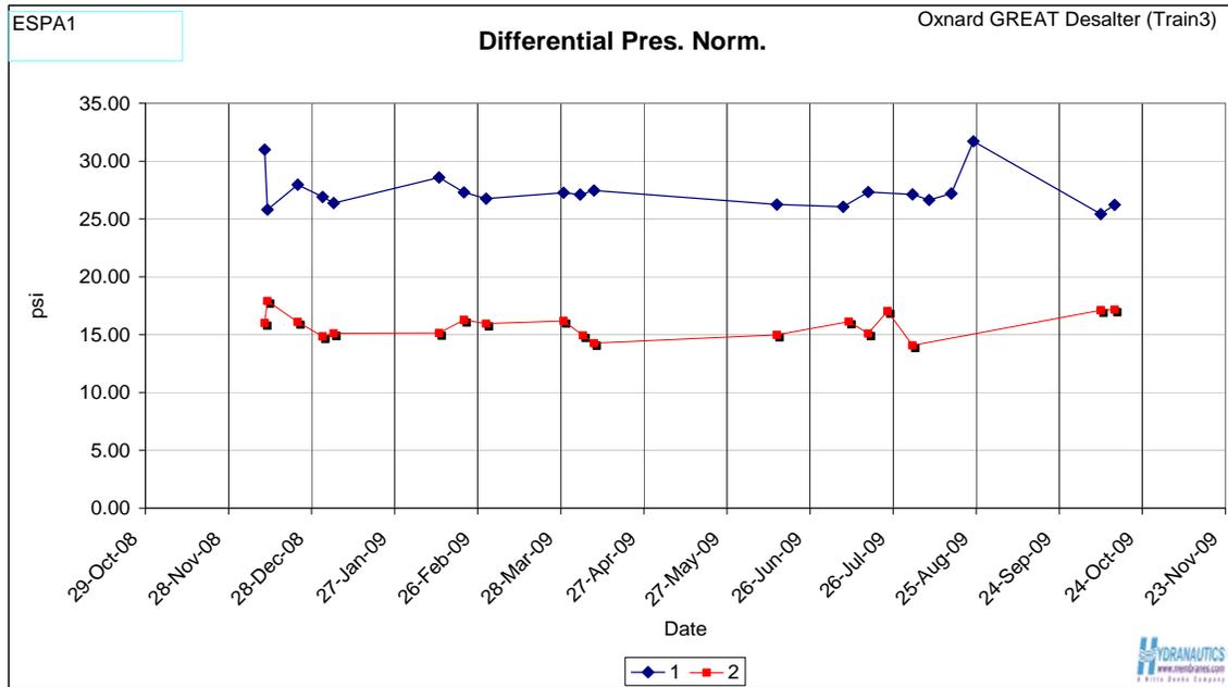
**Figure 10:** Differential Pressures of Oxnard Desalter Stage 1 and 2
