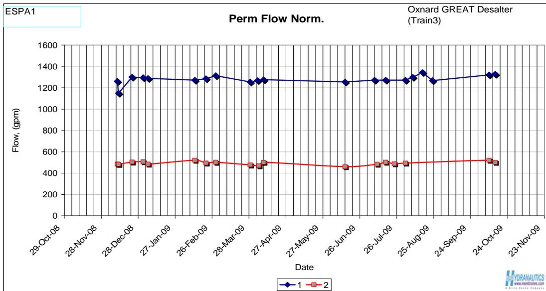
**Figure 9: Stable Normalized Permeate Flow over 1 year of operation**
