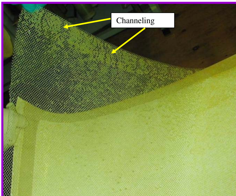
Figure 4 Fouled feedspacer from used element
