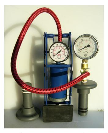
Example test apparatus with pump, pressure gauges, fittings, and adaptors. Parts are NOT sold by Hydranautics.
