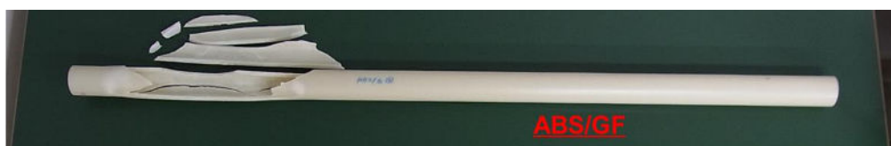
Figure 8. Permeate core tube collapse and mechanical failure.
