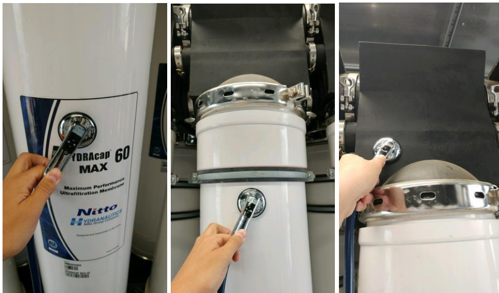
Figure 3: Stethoscope locations to check for bubbles on HYDRAcube module.
