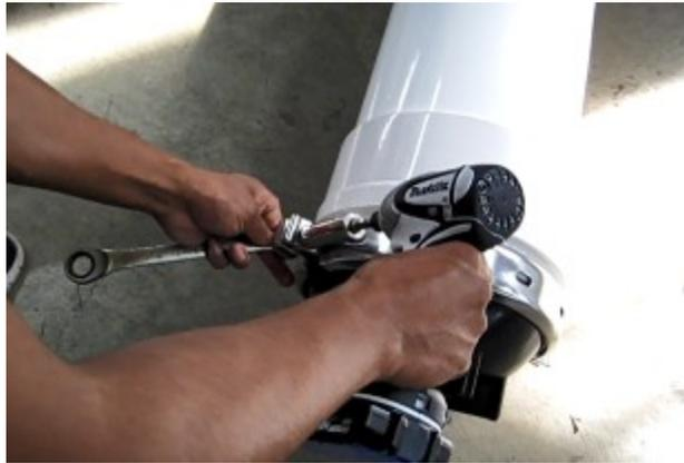
**Figure 2: Loosening of the end cap clamps.**
