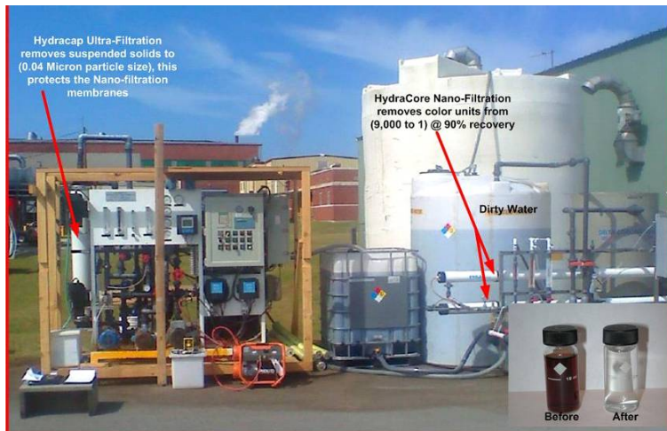
Figure 8 Pilot system for field testing of pulp and paper wastewater
