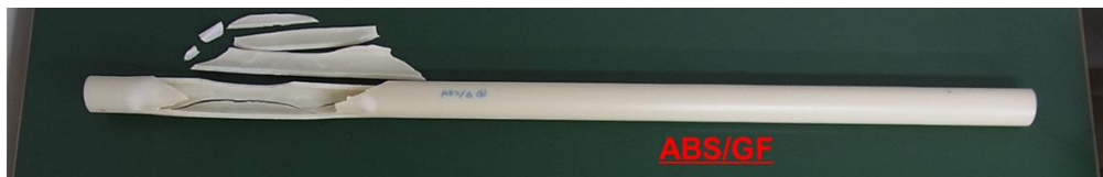
Figure 9. Permeate core tube collapse and mechanical failure.
