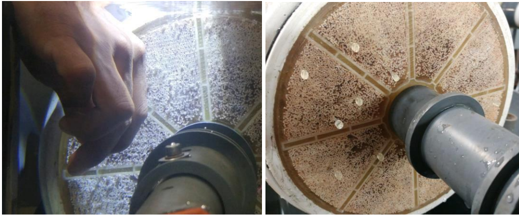
Figure 5: Temporarily installing pins into broken hollow fibers.
