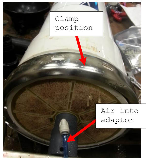
Figure 2: Clamp and air inlet locations.
