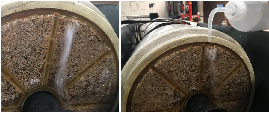
Figure 4: Air stream example using a bottle with water.
