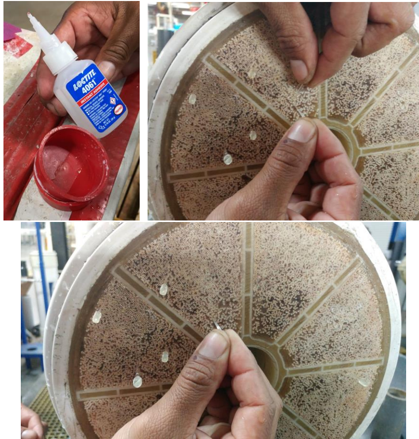
Figure 6: Permanently installing repair pins with Loctite 4061
