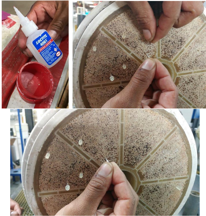
Figure 6: Permanently installing repair pins with Loctite 4061
