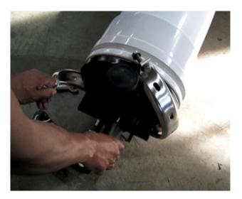
Figure 3: Removing the end cap clamps.
