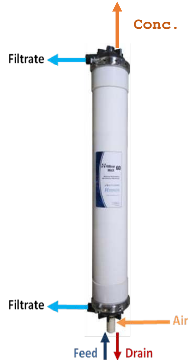
Figure 2: Module Components and Port Configuration
