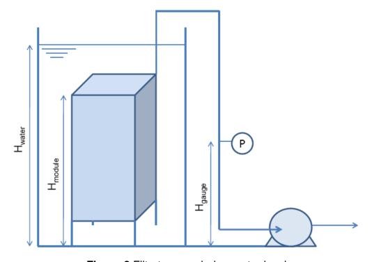
Figure 2 Filtrate pump below water level
