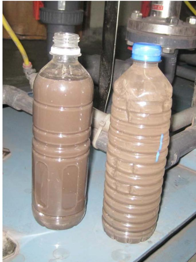
Backgrinding + Dicing WW (left) and Dicing WW only (right)
