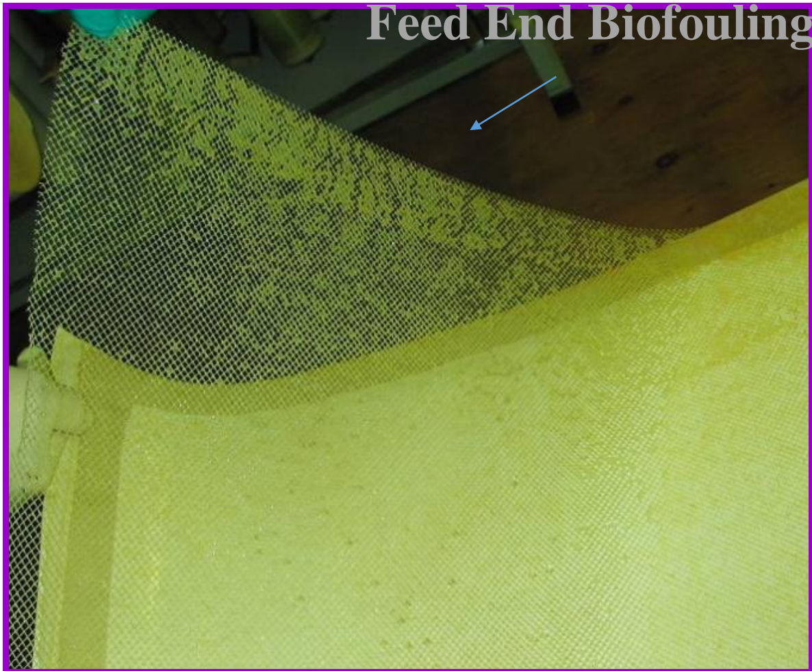
Photo 1 - Biofouling Formation at Feed End of RO Element
