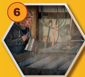
**6** The concentrated sap is boiled down to syrup in the evaporator and then sent for further inspection and grading
