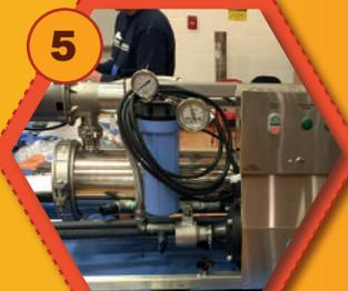
**5** RO membranes concentrate the sap by removing more than 90% of the water from it
