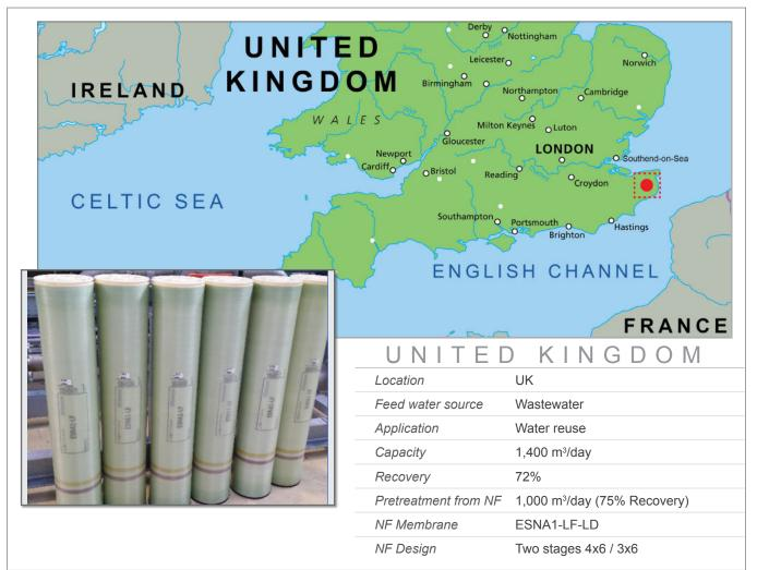
The fouling produced very high feed pressure in both stages of the NF system, while the differential pressures remained constant. Hydranautics' team visited the site for elements autopsy and recommended process modifications. Parameters of wastewater to be treated:
