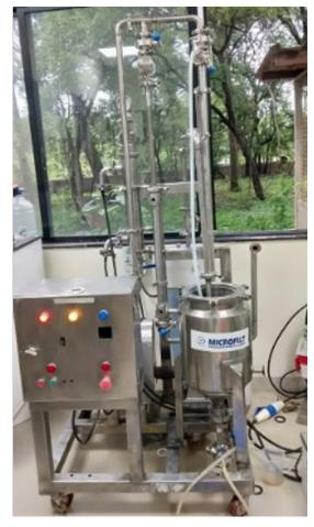
Figure 2: Picture of the lab-scale NF test unit
