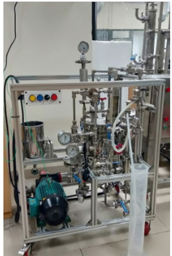
Figure 2: Picture of the lab-scale NF test unit
